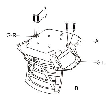
Then fix the armrest (G) with seat (A) by 4 x screws (3) and 4 x washers (7). Tighten all screws.
